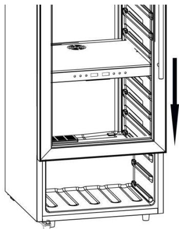
7. Relocate the upper hinge part at the left, and cover the right hinge hole with black pad
