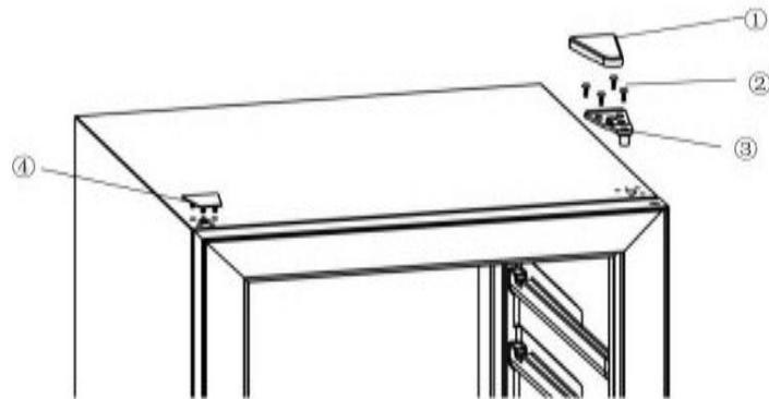
3. Remove the door from the cabinet by opening it slightly and lifting
