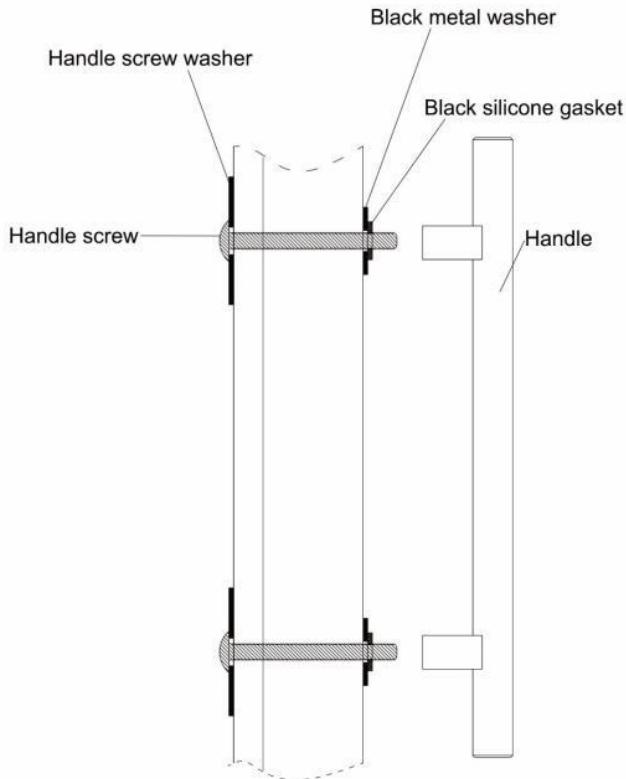
3. Align the handle with the screws and tighten the screws until the handle is aligned with the door and secured tightly against the door (DO NOT over-tighten as this will cause damage to the handle assembly and door glass surface).
