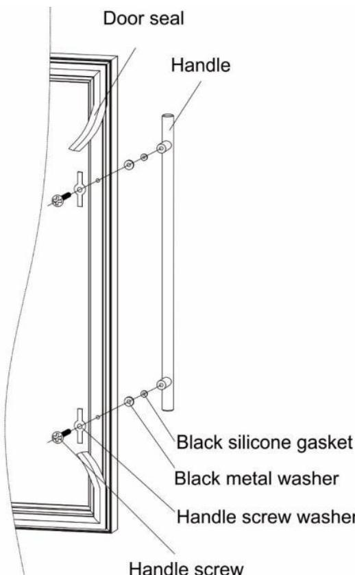
2. Follow below diagram to insert all handle installation accessories into handle fixation holes:
