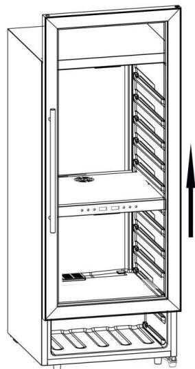
4. Remove the lower hinge parts at the right and then install it at the left
